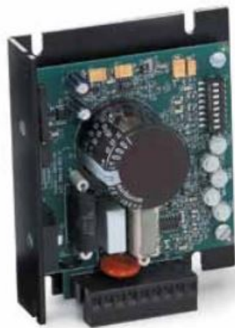
Figure 3.9: Speed Controller of Motor
